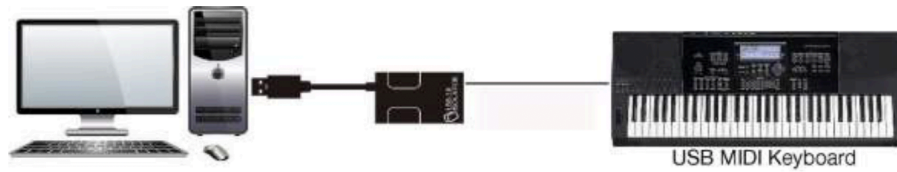
Fig 1. The USB Isolator unit is installed in-line between the PC and a connected USB device.
