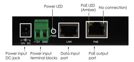
• DC-jack and 2-pin terminator blocks for power input: To inject the DC power to the Ethernet cable, the Injector needs a 12V DC power applied either on its DC jack or the 2-pin terminal blocks (but not both at the same time), its internal circuits will convert it to 48V DC to use for PoE.
