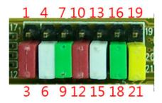
7 x 3 header block to enable Termination and BIAS resistors
