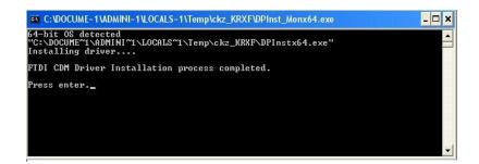
5. After the message "FTDI CDM Driver installation process completed" appears, press "Enter" to complete the driver installation.
