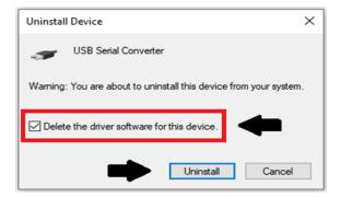
Note: If you have more than one USB Serial Converter installed in your PC, you need to repeat steps 8 - 10 to delete the driver software for each converter.
